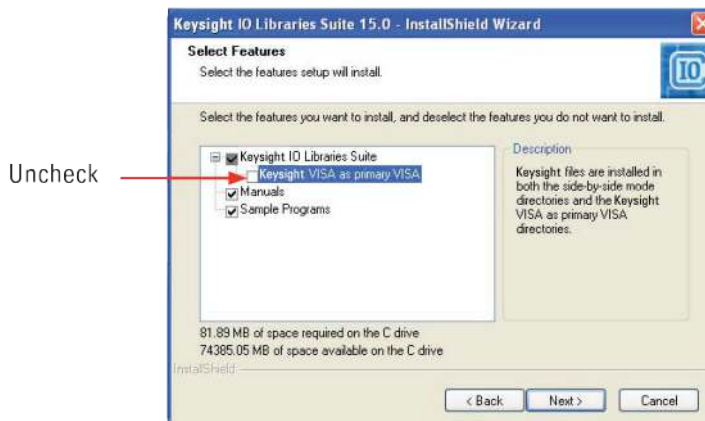
Figure 5. Enabling side-by-side mode in Custom setup
