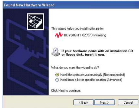
Figure 6. Installing the Keysight 82357B USB/GPIB
