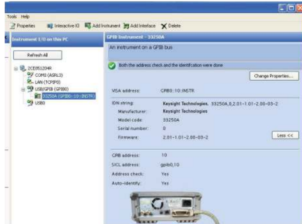
Figure 9. Connecting the USB/GPIB converter to the instrument
